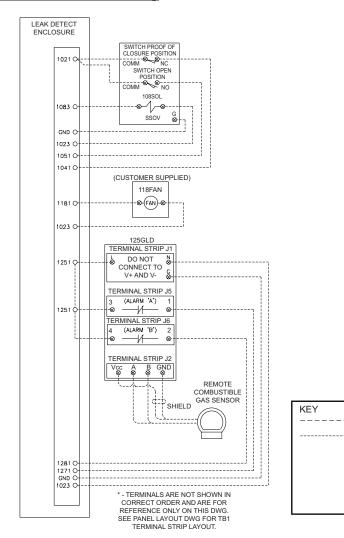
Eclipse external wiringCustomer field wiringTerminal block
